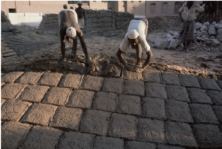
FIGURE 7.10 Mud Bricks Molds. CREDITS: CHRISTIAN DARLES.
