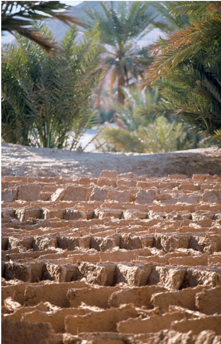
FIGURE 7.12 Drying Bricks arranged vertically for better Ventilation.
