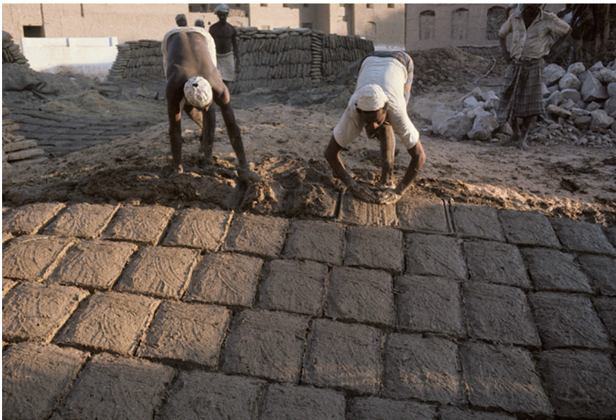
FIGURE 7.10 Mud bricks molds CREDITS: CHRISTIAN DARLES.
